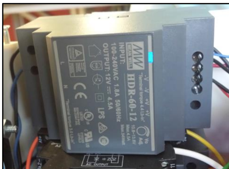
Figure S5. Using a precision screwdriver, the voltage on the 12 VDC and 24 VDC can be adjusted slightly (yellow circle). Turn clockwise to increase, and counter-clockwise to decrease.
